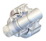
This dual pressurized, high-temperature metal bellows gas seal is engineered for the hottest process pumps found in refinery and hydrocarbon services. Qualification tested per API 682 Type C, Arrangement 3 requirements.
